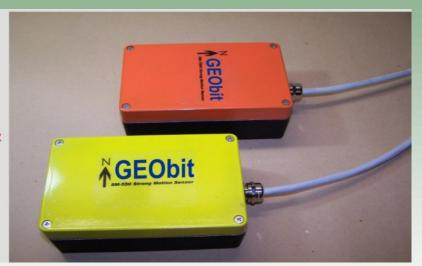
The SM550 and SM1500 are two MEMS type, three-component acceleration equivalent output sensor. Both have wide frequency response. Model SM1500 has a response from DC to 1500Hz, while the SM550 model has a response from 0.5 to 550Hz
