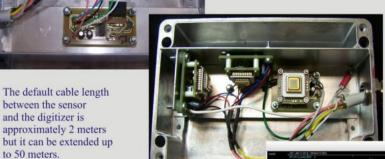
The SM1500 sensor operates from a bipolar power supply that can range from +/-6V to +/-15V with a typical power consumption of 33mA @6Vdc
